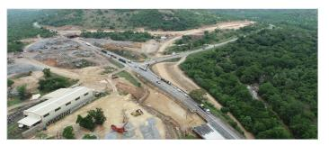
The N4 Montrose Interchange received its first upgrade in over 30 years, replacing an at-grade T-junction with a free-flowing intersection. Image courtesy of SMEC South Africa.
