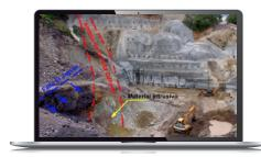
During the construction of a road in the Mexican state of Nayarit, a considerable mass of rock started sliding close to a tunnel portal, putting the construction site at risk. To find a solution, the team created a 3D model with PLAXIS to accurately represent the movement of the rock mass, as well as 2D PLAXIS cross sections to complement the 3D model. These models were used to calculate the new excavations, structures, and compacted fills of the project.
