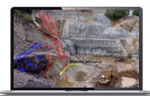
During the construction of a road in the Mexican state of Nayarit, a considerable mass of rock started sliding close to a tunnel portal, putting the construction site at risk. To find a solution, the team created a 3D model with PLAXIS to accurately represent the movement of the rock mass, as well as 2D PLAXIS cross sections to complement the 3D model. These models were used to calculate the new excavations, structures, and compacted fills of the project.
